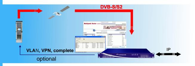
The satellite data receivers MediaSputnik 1022/1032 series receive IP the data in basically through the satellite and territorial DVB broadcast channels, organize return channels over accessible communication, including the synchronous and asynchronous channels. At connection of receivers to local area networks, IP packets are route to data transfer local network.
